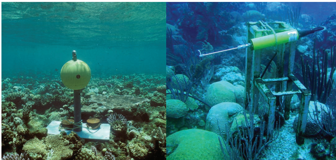
FIGURE 4. An InterOcean S4 electromagnetic current meter in place on a shallow reef, and a Sontek ADV flow meter on a stand that allows vertical profiling from just above coral tentacles to 2 m above the bottom. These and several other recently developed instruments have been used to characterize flow on coral reefs. Photos by Kenneth Sebens.
