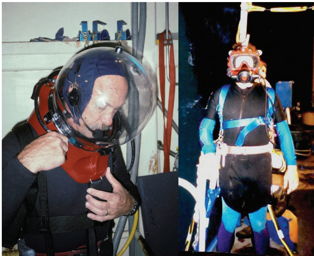
FIGURE 3. Full face mask (K. Sebens, 1999) and helmet (G. Wellington, Jason Project, 1996) systems supplied air from Aquarius (left) and from the surface barge above Aquarius (right). Photos by Kenneth Sebens (left) and Karla Heidelberg (with permission, right).
